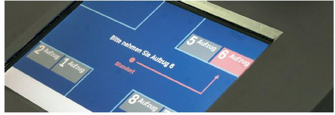
**Fig. 2** Destination Selection Control (DSC). The photo (©ThyssenKrupp) shows the indication of the elevator to be taken; cf. Figure 3 for a schematic view.
